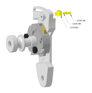
Replace the ratchet plate on the back of the casting using a 2.5mm Allen (hex) key
