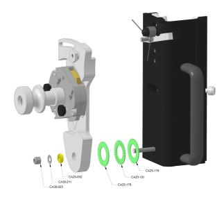
Clean and smear with petroleum jelly or lithium grease the two large washers and thrust bearing from the bottom end of the casting.
