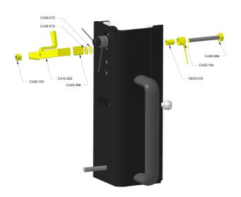
Remove the ratchet lever nut using an 8mm spanner/wrench and take off the ratchet lever and washer. Remove the long screw, spring and spacer from the back face of the carriage after first taking a photograph of the spring position for reference.
