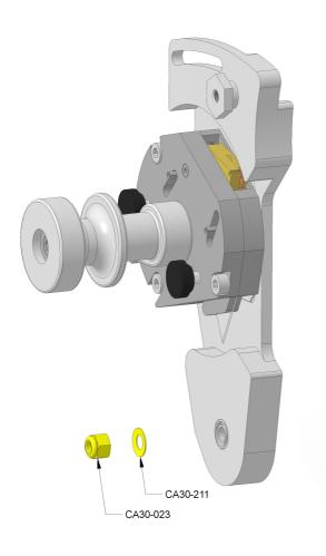
Replace the swinging arm casting over the two screws, press down on the ratchet lever to mesh the teeth. Replace the dish shaped washer with the orientation as before then replace and lightly tighten the nut with a 10mm spanner/wrench.
