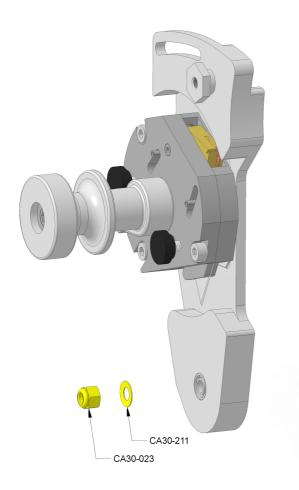
Remove the lower casting fixing nut and washer (note the washer's orientation) with a 10mm spanner/wrench.
