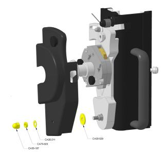
Remove the swinging arm casting.
