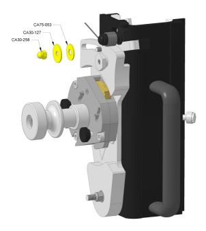
Remove the nut and washers adjacent to the curved slot in the casting using an 8mm spanner/wrench
