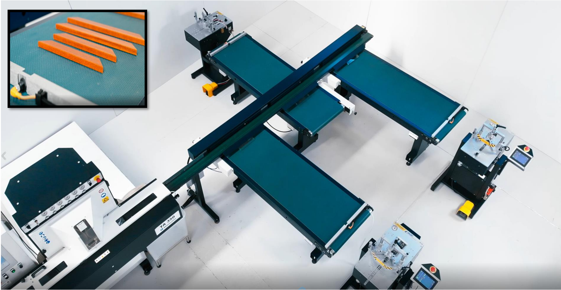
Electronic Exit Belts Sensor Control/Detect pcs overflow/status
