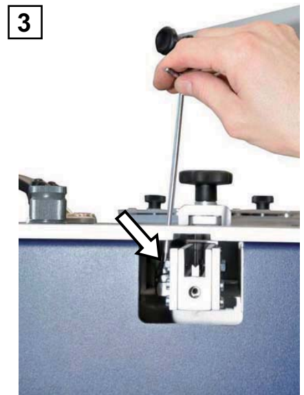
3. Remove the screw which secures the magazine to the pneumatic V-nail pusher actuator
