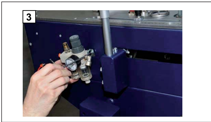
3. Secure the unit in place with the 2 socket head screws.
