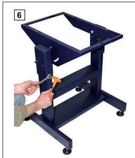
6. Tighten the grub screws and lock nuts.
