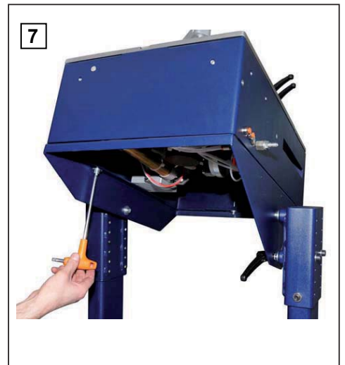
7. Position the machine on the cradle and fasten in place by inserting the 3 socket head screws as indicated by the arrows.
