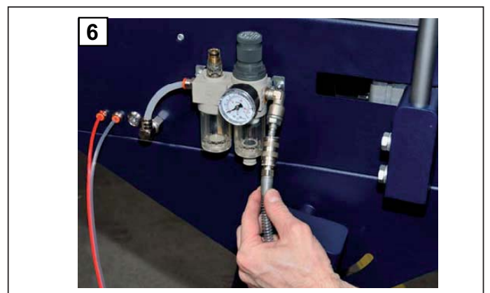
6. Connect the compressed air supply and adjust the pressure to at least 6 bar, checking this value on the gauge.
