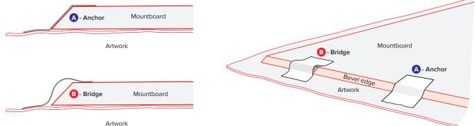
The paper is mounted on a piece of conservation grade mountboard which is bevel cut approx. 10mm all round smaller than the paper. The paper is then held in place with pieces of gummed paper tape. The same 24mm or similar gummed paper tape is used in three ways:
