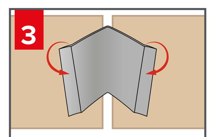
and the smaller wings twist out even further thanks to their specially engineered shape, unlike V Nails with straight wings.
