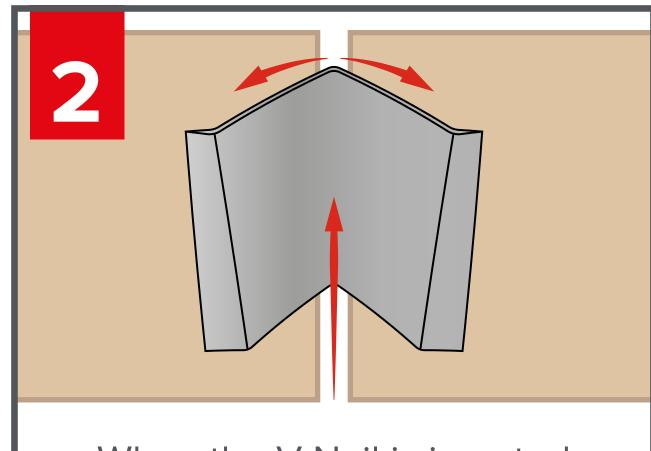
When the V Nail is inserted into the frame the large wings spread out...
