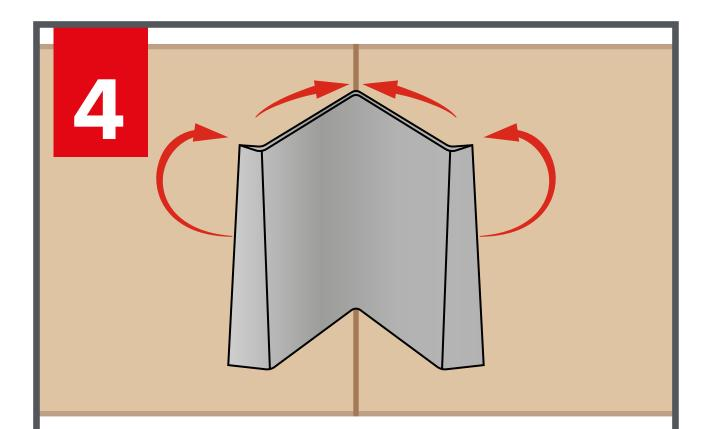
As both parts of the wing contract, the moulding is pulled closer together, making the corner join extra tight.
