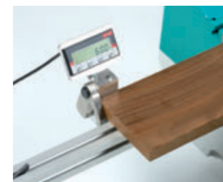
Digital display for flip stops
