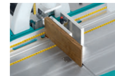
Butt stop fence elevation
