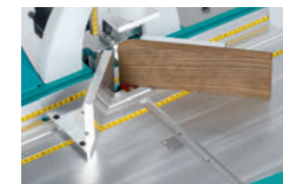
Internal fence elevation
