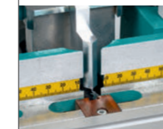
Centre line location jig
