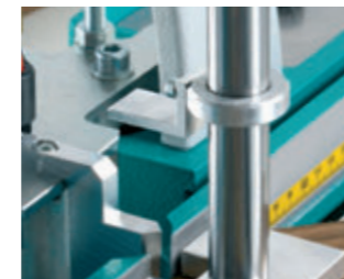
Routing depth and lever limiter
