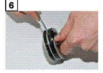
Remove the seals from the hammer, clean well and grease, check for wear or the presence of chips. Install the new seals making sure the lip seals are placed the right way round.
