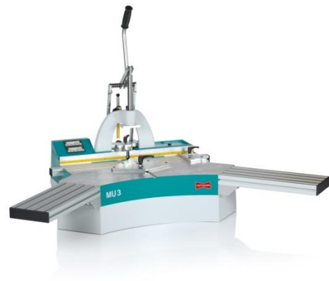
Hoffmann MU3-D manual dovetail routing machine (shown with optional accessories)
