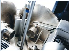
Pneumatic system for controlling the up and down movement of cutting saw blades
