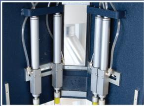
Inside cabinet view of adjustable pneumatic hold-down clamps
